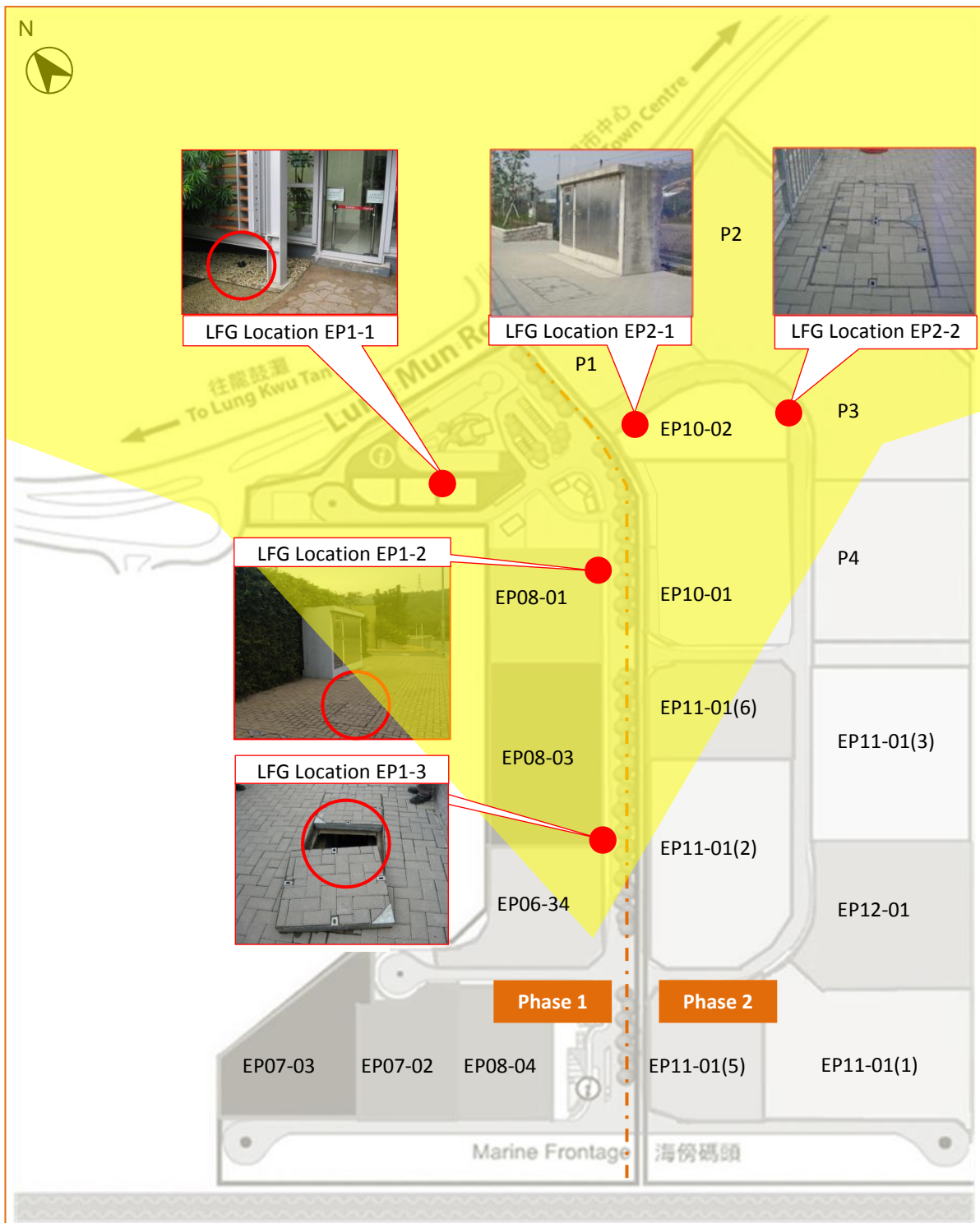
Figure 2-1 LFG Monitoring Locations Within EcoPark
