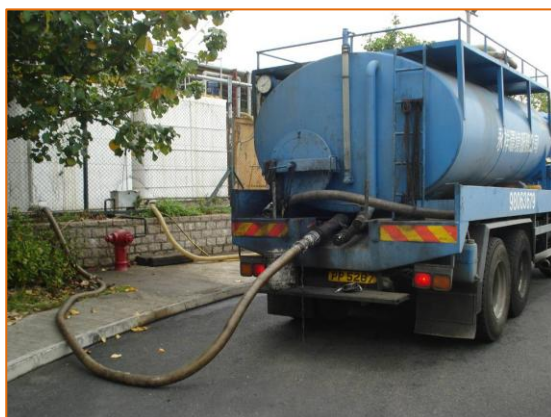
Photo 2 Transference of Oil/Water Mixture from Tanker to Oil/Water Mixture Storage Tanks
